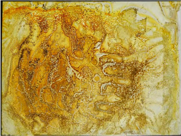
Fig. 8: Chemically disintegrated glass plate of the nebula NGC 3115 (Sextantis), taken with the Mount Wilson 60-inch reflector, December 23, 1911, exposure time of 100 minutes, reproduced with permission of the Royal Astronomical Society.
